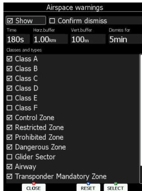
Airspace Warning Setup
